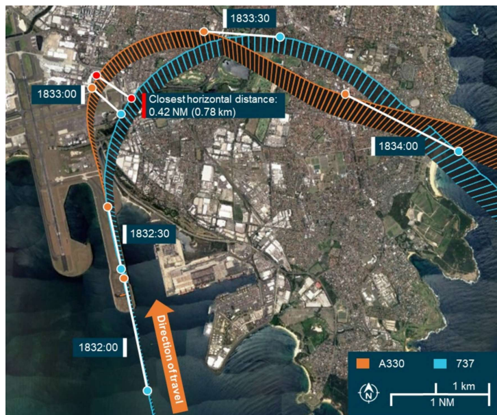
Actual paths on the night with white lines showing space between the aircraft at particular points in time (source: ATSB).
